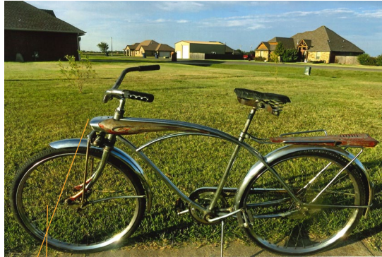
Figure 2: Showing the castor distance \delta on a 1994 Kawasaki Vulcan (top) and a 1962 J.C. Higgins Flightliner (bottom). Their front wheels have been deliberately set straight ahead. Photos by Dwight E. Neuenschwander.
