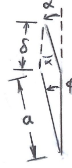
Figure 7: Turning the front wheel through angle \alpha turns the bike frame behind the steering axis through the smaller angle \varphi in the same sense.
